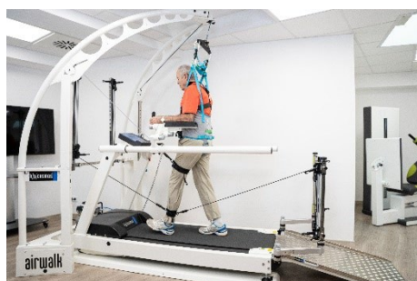
Figure 40. Single-sided installation of the robowalk® active gait trainer in support mode.
